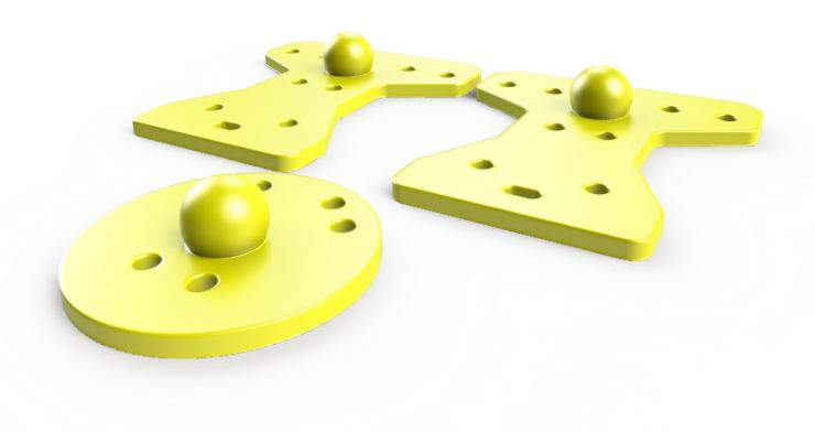
Bogert Aviation's Lear Jet Jack Pad Kit includes heavy duty jack pads for most Learjet Aircraft. Made from 1/4" steel plate and 1" diameter jack points, powder coated for high visibility. Compatible with most floor jacks.
