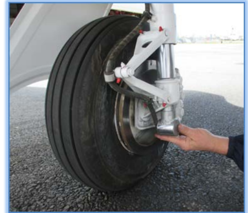
FIGURE 1: PAD WILL EASILY FIT INTO THE BARREL OF STRUT. DO NOT FORCE.
