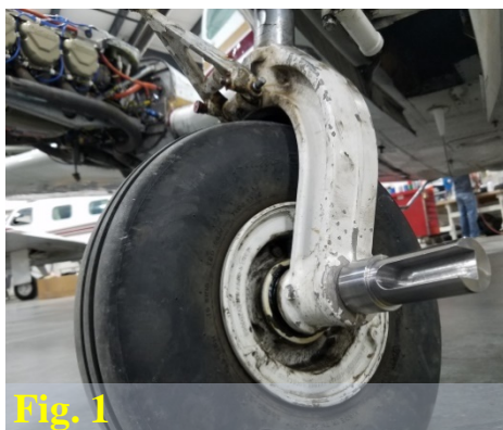
Axle Pin 30M-B35/58-P shown with Bottle Jack Adapter 30M-B35/58-A .
