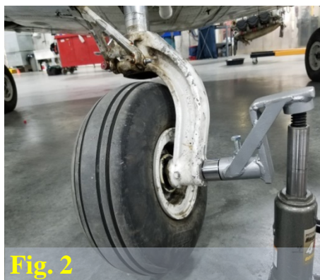
Axle Pin 30M-B35/58-P shown with Bottle Jack Adapter 30M-B35/58-A .
