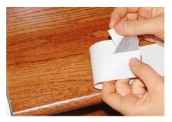
**3.** Roll back the left edge of No-*Slip* Tape and peel back the right half of the release liner as shown above to expose a small portion of adhesive.
