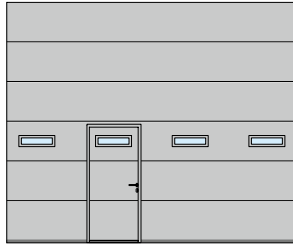
SPU F42, SPU 67 Thermo Type D section windows Wicket door arrangement on the left
