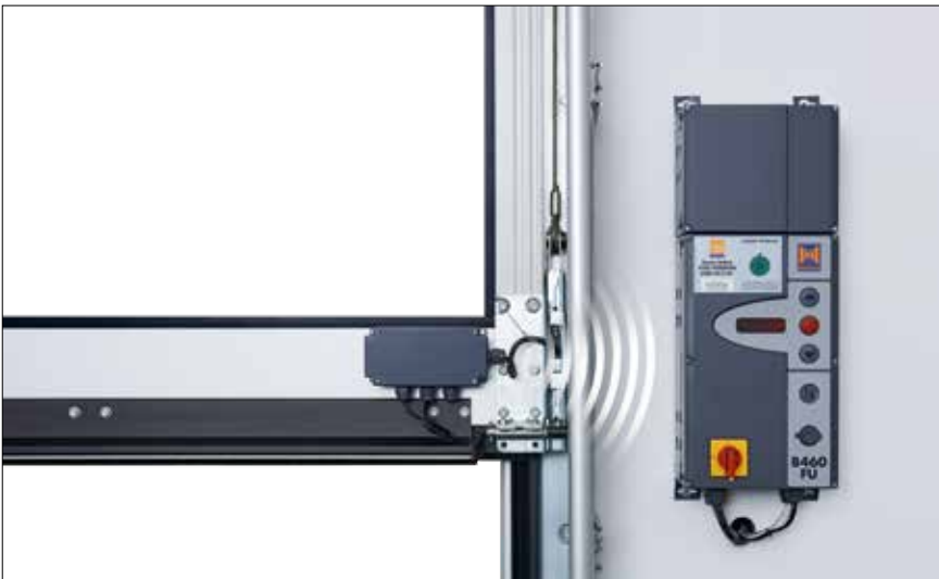
Radio transmission unit To transfer the signals from the door leaf to the control via Bluetooth (no coiled cable), power supply via a powerful battery; connectable components: optosensors LE (low energy), leading photocell VL 1-LE / VL 2-LE, 8k2 strip, cable slack switch, wicket door contact, night latch contact For all controls
