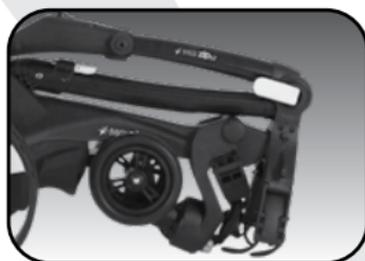
**Step 5:** Push the toggle down on the top bag support and then move the Top Bag Support down so that it locks over the front wheel assembly.
