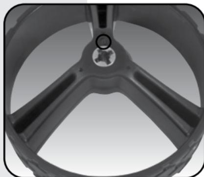
**Step 2.** On the wheel, press the grey release button on the wheel hub. Place the wheel onto the axle. You will notice you need to match up the inner female groove on the axle and the male of the wheel. When placed in position simply release the button. You will notice you hear a "click" when the wheel is properly secured. To check that the wheel is properly in position pull on the wheel. If it is properly in position it will not slide off. Repeat for the other wheel.
