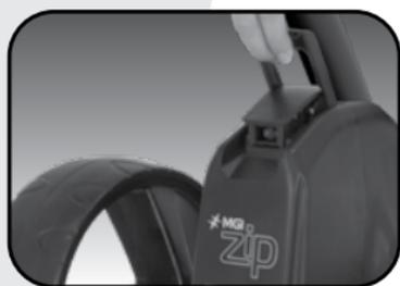
**Step 1:** Disconnect the battery by lifting the battery handle. It can be left on or removed from the Zip X2.
