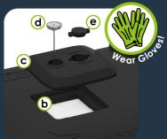
Place the filter bag (b) into the lid recess, fit the lid panel (c) front edge first then situate the thermometer (d) and valve (e).
