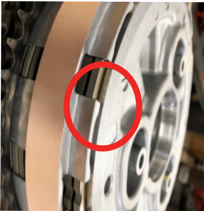
Photo #1. Fully Seated and ready to install springs.
