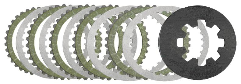
This kit consists of 5 friction, 5 steel plates and a 15% stronger than stock diaphragm spring. Plates should be pre-soaked in the same fluid you will be using in the bike for about 10-15 minutes. The type of fluids we recommend are any HD petroleum based, non-synthetic, primary oil, as light weight as possible, or even a good petroleum based motor oil such as 10/40 or 20/50 in weight. You can even use ATF Type F or B&M Trickshift.
