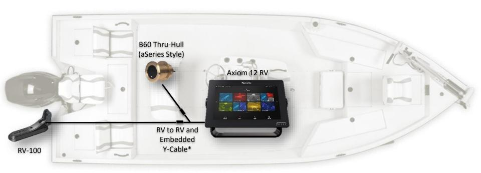
\*With the y-cable, you lose the ability to operate the conical sonar channel on the RV-100, instead electing to see the 50/200kHz channel of the P79
