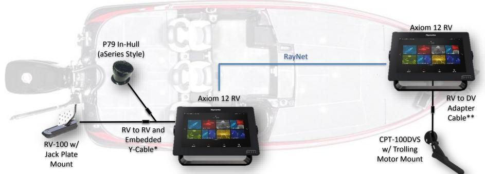
\*With this y-cable, you lose the ability to operate the conical CHIRP sonar channel on the RV-100, instead electing to see the 50/200kHz channel of the P79 \*\*DownVision and conical CHIRP sonar channels only
