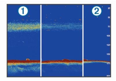
You can use echo stretch and filter width together to obtain the preferable resolution and noise reduction. With echo stretch and filter width set to low, the display has the highest resolution, but is the most susceptible to noise. With echo stretch set to high and filter width set to low, the display has a lower
