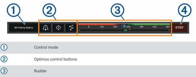
You must press a mode button on the overlay bar to engage or disengage the mode. When the mode is engaged, the button is illuminated.
