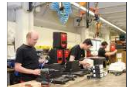
Final assembly of switch cabinets
