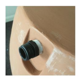
1) Apply PTFE tape to the finer thread on the Adaptor Nipple & Screw into the Barrel.
