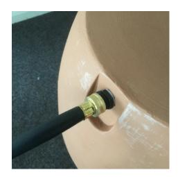
2) Screw the female end of the hose onto the coarser thread of the Nipple.
