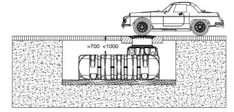
Coverage heights with cast telescopic dome shaft with cast iron lid or Begu (with cover class B respectively D - to be provided at construction site). Maximum load of the area used by passenger cars 3,5 to.
