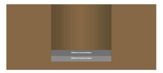
13.2. Place chamber in the center of the excavation and position firmly into the damp concrete base. Ensure the chamber is level and in the correct position.
