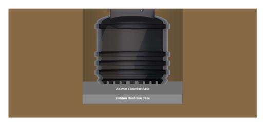
13.3. Fill chamber with a minimum of 700mm water in readiness for the first concrete pour.
