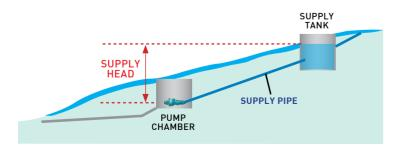
If the Spring/Stream is on a steep gradient you can achieve a good Supply Head within a small distance. In this case, water can be fed directly to the Supply Tank.
