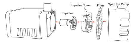
If after some time the pump starts losing power or stops working you should check for the build up of sediment or scale in the filter or in the pump housing. The filter housing can be removed by pressing down on the bottom of the filter housing.
