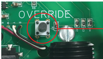
Figure 8 Solenoid Bypass Button
