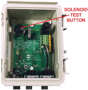
Figure 3 Solenoid Test Button
