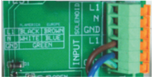
Figure 2 Wiring Colour Guide
