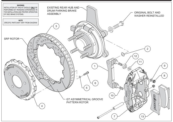
Figure 1. Typical Installation Configuration
