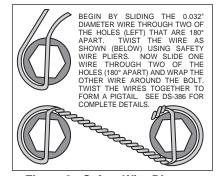
Figure 3. Safety Wire Diagram
