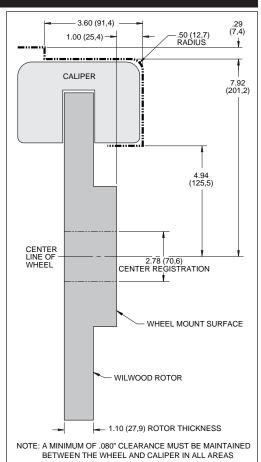
Figure 2. Wheel Clearance Diagram
