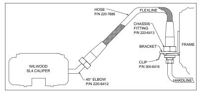
Figure 4. Brake Line Diagram
