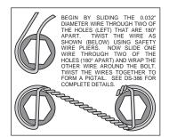
Figure 3. Safety Wire Diagram
