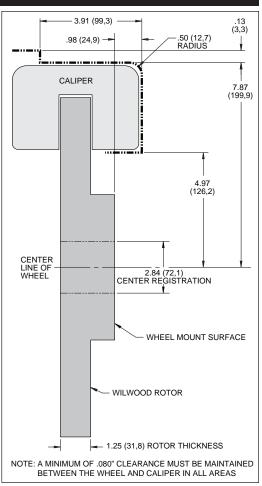
Figure 2. Wheel Clearance Diagram
