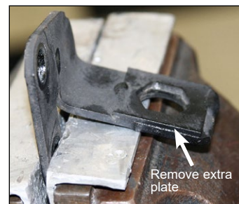
Photo 8 Before Plate Removal
