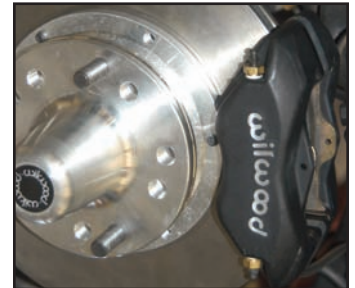
Photo 11 Caliper Bleeding Position
