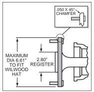
Figure 3. Axle Flange Maximum Dimension
