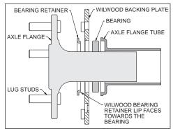
Figure 4. Retainer / Axle Diagram
