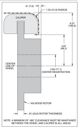
Figure 2. Wheel Clearance Diagram
