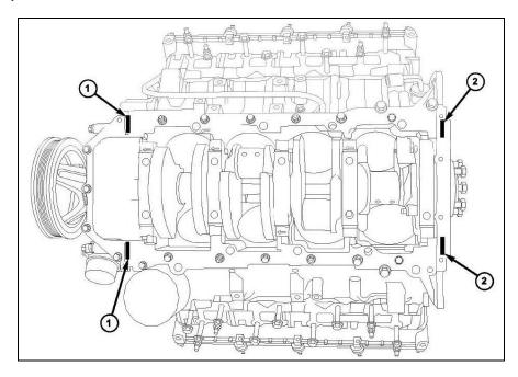
10. Position the windage tray to the engine block. Install the oil pump pickup in the oil pump housing per manufacturer's instruction. **IMPORTANT: Use O-ring included with the new pickup tube only.**
