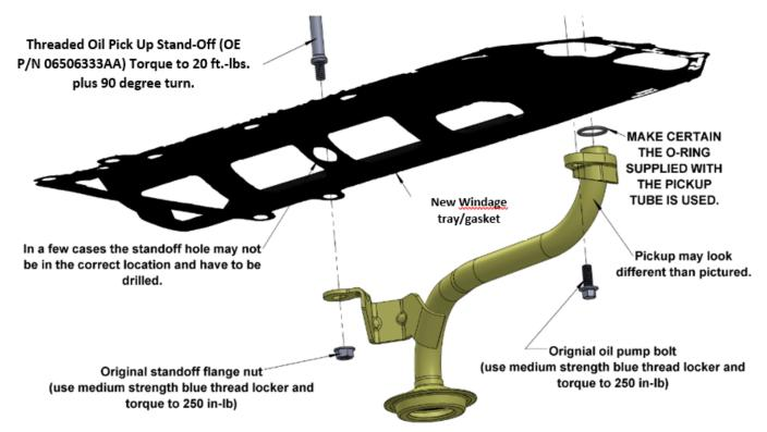
11. Position the pan onto the engine flange. Install all oil pan bolts by hand while ensuring the bolts thread in easily. Using a 10mm socket, follow the below sequence and tighten each of the M6 bolts, first to 106 in./lbs. **DO NOT OVERTIGHTEN THE PAN BOLTS!**
