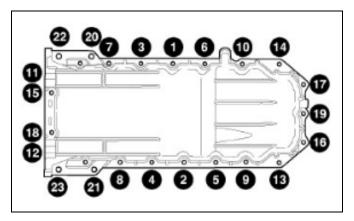
Note: Do not pry on the oil pan or oil pan gasket. The oil pan gasket is integral to the engine windage tray and does not come out with the oil pan.
