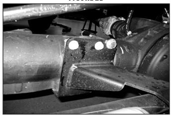
5. Remove the tie rod adjusting bolt and rotate the clamp 180 deg so the bolt is on top. Reinstall the bolt from front to back for stabilizer clearance. (Fig 3)
