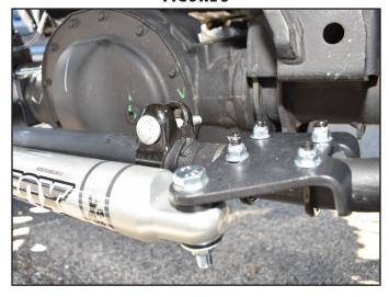
6. Install the driver's side stabilizer bracket to the top side of the tie rod end. Measure the distance between centers of the stabilizer mounts and set the same as the passenger's side. Tighten u-bolt hardware to 20 ft-lbs. Do not over torque, or the bracket may become deformed. (Fig 4)
