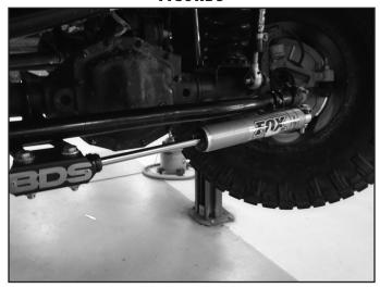
Failure to follow the proper installation location will result in damage to the steering stabilizers under full compression travel.
