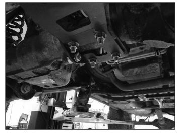
8. Attach the driver's side stabilizer bracket to the bottom side of the tie rod next to the clamp (Fig. 2) with the provided 5/16" U-bolts, washers, and nuts so the stabilizer mounting hole offsets to the outside. Leave hardware loose. Bolt Pack 304
