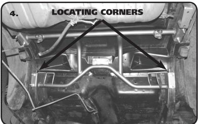
**4.** Install the cradle into the car. The rear corners of the Upper Bar Mounts locate into the front corner of the factory shock sheet metal mount. The Cradle is held in by (7) 3/8" Square U-bolts. Use the Cradle as a locator for drilling the holes. Drill the holes using a 7/16" drill bit. Drill The front 3 holes on each side with a 5/16" drill bit.
