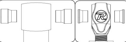
New R-Joints will be quite stiff (75-90 in/lbs breakaway torque) until they "break in" after a few miles of use. After the break in period they will move much more freely. Because the composite bearing race contains self lubricating ingredients, no additional lubrication is needed or desired. Any additional lubrication will only serve to attract more dirt and debris to the R-Joint and actually shorten its life.
