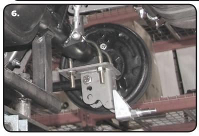
**6.** Install the Lower Axle Mount onto the Axle using the supplied U-Bolts. Run the nuts down to hold the mount in place, but DO NOT tighten yet.
