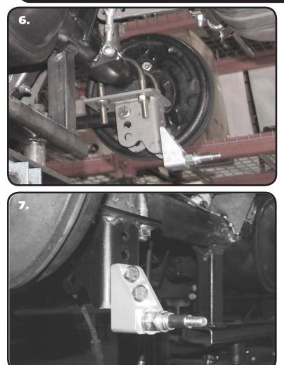
**6.** Install the Lower Axle Mount onto the Axle using the supplied U-Bolts. Run the nuts down to hold the mount in place, but DO NOT tighten yet.
