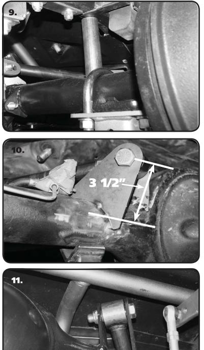
**9.** One helpful trick to maintain ride height when setting the pinion angle is to put a spacer between the axle and the frame. The spacer should be 4 1/2" tall. Set the pinion Angle and axle center. When measuring the axle center you can measure off of the frame rails. We also use a plum bob off the quarter panels to double check the axle center. Refer to Page 6 on Setting the Pinion Angle.
