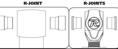
New R-Joints will be guite stiff (75-90 in/lbs breakaway torgue) until they "break in" after a few miles of use. After the break in period they will move much more freely. Because the composite bearing race contains self lubricating ingredients, no additional lubrication is needed or desired. Any additional lubrication will only serve to attract more dirt and debris to the R-Joint and actually shorten its life.
