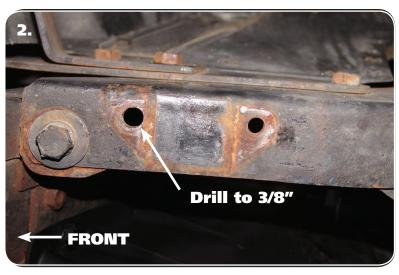
**2.** Drill Out the forward ORIGINAL swaybar mounting hole to 3/8" The original rear hole will not be used. A new mounting hole for the rear bolt will be drilled in Step #4.
