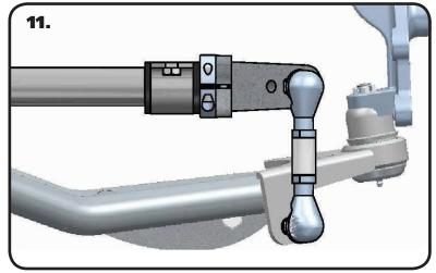
**11.** With the arms installed on the MuscleBar, install a 3/8" Flatwasher on each side of the tab along with a 10mm Nylok Nut onto the Posilink and Tighten.
