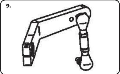
**9.** Install the Posilink into the center hole on the MuscleBar arm using Diagram #7 as a reference. Tighten using a 3/8" Flatwasher on each side of the arm and a 10mm Nylok nut.
