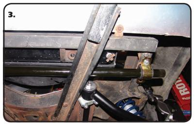
**3.** Insert the MuscleBar into position by sliding it between the bumper support and the frame rail. With the MuscleBar slid in place, install the mount bushing onto each end of the MuscleBar followed by the mounting strap.
