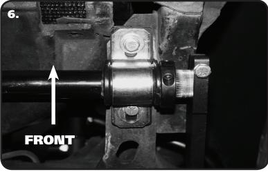
**6.** The MuscleBar will be slid to the rear of the car when doing final tightening of the Bushing Mounts.
