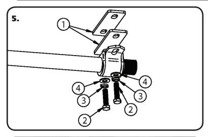
**5.** The Musclebar on the C3 is bolted into the OEM swaybar position. The C3 uses Spacers(1) to position the bar correctly on the chassis. These spacers are installed in between the Bushing Assembly and the frame. Insert a 5/16" x 1 1/2" Bolt(2), 9/16" Lockwasher(3), and 5/16" Flatwasher(4) through each slot in the Bushing Mount. Install the 2 Spacers(1) on the bolt before threading it into the factory swaybar mounting hole in the frame. **DO NOT TIGHTEN.**
