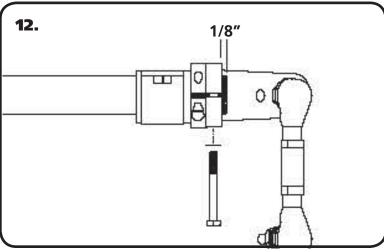
**12.** Position the Arm so that it is inset 1/8" from the ends of the splines. Install 5/16"x 1 3/4" bolt, along with a 5/16" Lockwasher in from the bottom of the MuscleBar arm. **Torque the bolt to 35 ftlbs**.
