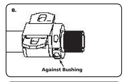
**8.** With all 4 bolts installed, center the MuscleBar in the bushings. There should be approximately (1 3/8"C2) (1 9/16"C3) sticking out of the bushing on each side. With the MuscleBar center, slide the locking rings up against the bushings and tighten them down. Tighten the Bushings Mounting hardware.
