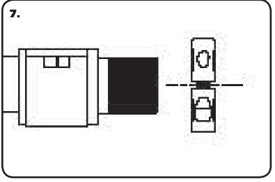
**7.** Install locking ring onto MuscleBar. **DO NOT TIGHTEN.**
