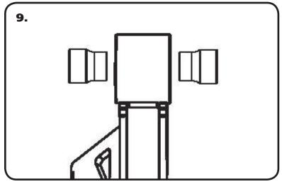
**9.** Install the 7/16" I.D. T-bushings into the front Trailing Arm Bearings. Do this for both Trailing Arms.
