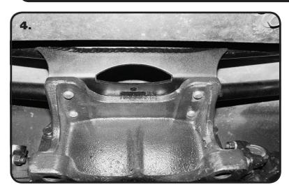
**4.** Attach the Upper Crossmember to the OEM Center Section using (4) 7/16"-14 x 1 1/4" Hex Bolts, (4) 7/16" Lock washers, and (4) 7/16" SAE Flat washers.
