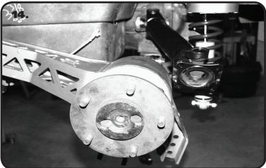
**14.** Reinstall the OEM Half Shafts using the OEM hardware.
