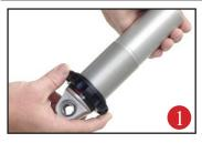
First using the supplied lower adjuster nut(90002222) thread the nut onto the shock from the bottom side as seen in figure 1.
