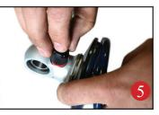
Once the knob is removed slide the Derlin washer over the spring, Next slide the upper spring mount (90002222) over eyelet as seen in figure 4.
