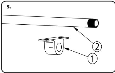
**5.** Install the MuscleBar Bushings and Straps on the MuscleBar. They are positioned approximately - **5"on C2**, **3 1/2" on C3** - from the end of the MuscleBar to the outside edge of the bushing. To install the Bushing, remove the Mounting Strap from the Bushing. Open the Bushing at the slice on the edge of the Bushing. Slide the Bar through the slice. Reinstall the Mounting Strap.
