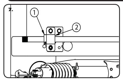
7. Center the bar by measuring from the edge of the Bushings to the end of the bar. With the bar centered, tighten the Bushing Assembly hardware. Install a Locking Collar(1) on each end of the MuscleBar(2). Slide the Locking Collars against the Bushings and Tighten the Collar.
