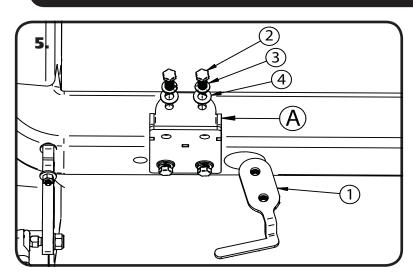
4. Insert the Nut Plate with Tab(1) through the large hole in the crossmember and line it up with the holes drilled in the previous step. Thread a 3/8" x 1 1/2" Hex Bolt (2), with a 3/8" Split Lock washer(3), and 3/8" Flatwasher (4) installed on the Bolt, into each bottom hole. Tighten both bolts. Do this for both sides
