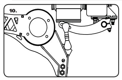
**10.** With both arms clocked, the Posilinks can be permanently attached to the StrongArm. Install a 3/8" Flatwasher on the Threaded Stud of the Posilink, insert the Stud into the Arm. Install a 3/8" Flatwasher and 10mm Nylok Nut onto the Stud and tighten.
