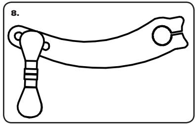
**8.** Install a PosiLink Assembly into the center hole one each MuscleBar arm. **Install the Posilinks in opposite sides of the 2 arms.** Install a 3/8" Flatwasher on the Threaded Stud of the Posilink, insert the Stud into the Arm. Install a 3/8" Flatwasher and 10mm Nylok Nut onto the Stud and tighten.
