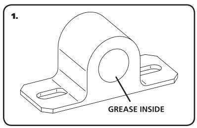
**1.** Apply Lithium grease to the inside of the sway bar bushings using the tube of grease supplied in the kit.
