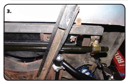
**3.** Insert the MuscleBar into position by sliding it between the bumper support and the frame rail. With the MuscleBar slid in place, install the mount bushing onto each end of the MuscleBar followed by the mounting strap.
