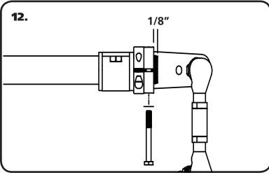
**12.** Position the Arm so that it is inset 1/8" from the ends of the splines. Install 5/16"x 1 3/4" bolt, along with a 5/16" Lockwasher in from the bottom of the MuscleBar arm. **Torque the bolt to 35 ftlbs**.
