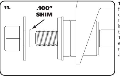
**10.** With the cross shaft tightened against the front bushing/inner sleeve, use the supplied shims to determine how much shim is needed to fill the gap. Typically, 1 or 2 shims will be needed. Hold the shim up to the gap to see how much is needed.
