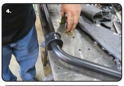
**4.** Open up the Poly SwayBar Bushings and install them over the Delrin Sleeves.
