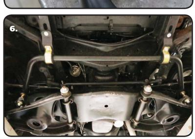
**6.** Hold the SwayBar into position on the truck with the SwayBar arms below the tie rods. Align the holes in the Bushing Straps with the holes in the Frame Brackets. Install a 3/8" Flat Washer on (4) 3/8"-16 x 1 1/4" Hex Bolts and insert them into the holes. Install a 3/8" Flat Washer and 3/8"-16 Nylok Nut on each Bolt. Center the bar in the bushings before snugging up the hardware. Do **NOT** completely tighten the Hardware. It will be left partially loose until the End Links are installed.
