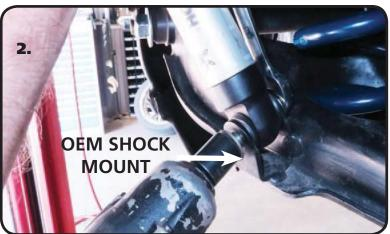
**2.** Attach the bottom of the Shock in the OEM location using the 1/2"-20 x 2 1/2" Bolt, Nut & Flat Washers supplied in the kit. The Lower Shock is Bolted to the Lower OEM Mount using the supplied Shock Sleeve.
