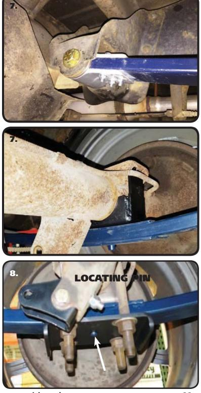
**6.** Swing the front of the Leaf Spring up into the front Hanger aligning the Differential with the Flip Bracket. It may be necessary to raise the Differential up to get the Leaf Spring into the front hanger. Align the holes in the Hanger with the Bushing Sleeve. Install a 9/16" Flat Washer on a 9/16"-12 x 4 1/2" Bolt supplied in this kit. Insert the Bolt/Washer through the Hanger & Leaf Spring. Install a 2nd 9/16" Flat Washer & 9/16"-12 Nylok Nut on the Threads sticking through.
