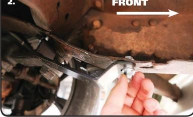
**1.** Some trucks are equipped with a sway bar. If your truck has one, the OEM mount will need to be removed to install the Street-Grip Sway Bar. This is done by removing the rivets. The rivets can be removed by chiseling the heads off and driving them out or by drilling the rivets out. The new Frame Mount bolts directly in place of the old mount. If your truck doesn't have a sway bar, the mounting holes will still be in the frame.
