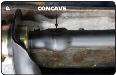
**8.** Reattach Control Arms to Truck. Use the OEM Hardware to attach the Lower making sure the Locating Pin for the lower cross shaft is in the hole. The Pin in the Cross Shaft Saddle will locate into the Holes. The Upper Control Arm Cross Shaft has a Concave area around the bolt hole. This Concave needs to go against the Convex Spacer on the Cross Shaft Bolts. The shims go behind the convex spacer. Reattach the Upper Control arms using the OEM Hardware and installing the Alignment Shims.
