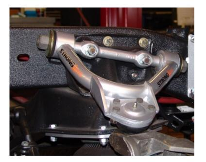
1. Drop the ball joint down through the upper control arm plate. Fasten to the arm w/ the hardware supplied.
