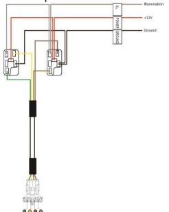
**Illumination (Gray)** - This wire provides power to the switch lights. It should be hooked up to a light circuit in the vehicle (dash lights) or it can be hooked up to a 12 volt switched source.
