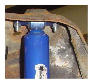
1. Attach the upper T-bar to the frame in the oem location using the supplied 5/16 x 1" USS bolts, washers and Nylok nuts.
