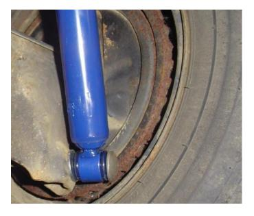
2. Attach the shock to the axle using the new cantilever pin supplied.
