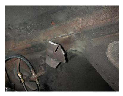
3. One more thing needs to be removed before starting the assembly; it's the pinion snubber and mount. For a clean cut use a cut off wheel and smooth any burrs.
