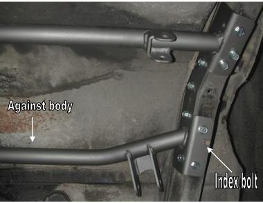
4. Lower the axle enough to slide the upper cradle into place. On most cars the location of the cradle will index off of the factory bump stop bolt hole. If your car has the bump stop beside the frame, slide the cradle forward until the front tube touches the body.
