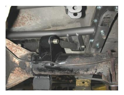
6. The heim end bar setup is designed to be offset to the inside of the car. The bolt hole in the mounting bracket has to be drilled out to 5/8" and the new longer bolt is used. The wider spacer is used on the outside with a narrow spacer on the inside. The bar is offset to provide better wheel and tire clearance.
