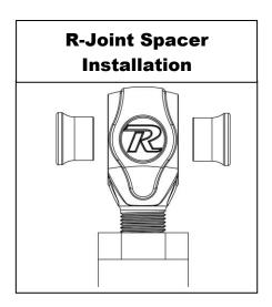
New R-Joints will be quite stiff (75-90 in/lbs breakaway torque) until they "break in" after a few miles of use. After the break in period they will move much more freely. Because the composite bearing race contains self-lubricating ingredients, no additional lubrication is needed or desired. Any additional lubrication will only serve to attract more dirt and debris to the R-Joint and actually shorten its life.
