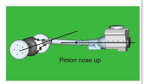
13. How do you set the pinion angle? On a single-piece shaft you want to set it up where a line drawn through the center of the engine crankshaft or output shaft of the transmission and a line drawn through the center of the pinion are parallel to each other but not the same line.
