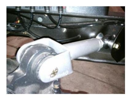
4. Fasten the other end of the bar to the axle using a  $\frac{1}{2}$ " x 3  $\frac{1}{2}$ " bolt and Nylok nut.
