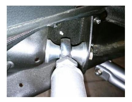
1. The length of the upper bar should be set from the factory at 10.26" center to center. Ensure that the jam nut is tight.
