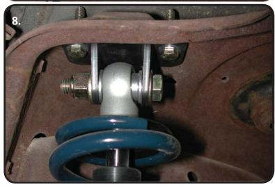
**8.** Fasten the CoilOver to the upper bracket using a ½" x 2 ½" bolt, 1/2" flat washer, and Nylok nut. ½" I.D. aluminum spacers must be installed on each side of the bearing. Torque to 75 ftlbs.
