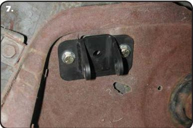
**7.** Fasten the new upper shock bracket into the factory shock location using the 5/16" x 1 1/4" bolts, flat washers and Nylok nuts supplied. Torque to 17 ftlbs.
