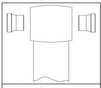
Insert the SMALL end of the spacer INTO each side of the center pivot ball. Push the spacer in until it bottoms out in the center pivot.
