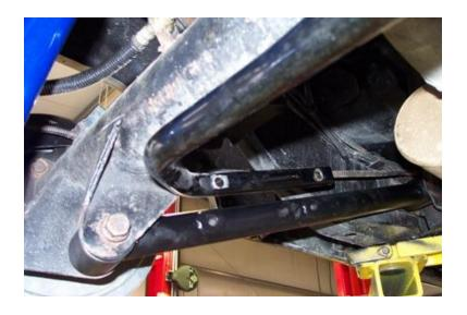
5. Attach to rear of the lower StrongArm to the frame using the ½" x 3 ½" bolts and Nylok nuts supplied.
