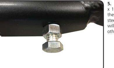
**5.** Thread the 3/8"-16 nut onto the 3/8"-16 x 1 ¼" bolt. Thread it into the front hole of the ball joint plate. You will need to adjust the steering stop to suite your needs. This setting will vary depending on wheel and tire size and other suspension components.
