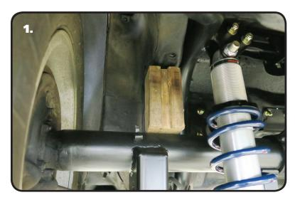
**1.** One helpful trick to help maintain ride height while setting up the rear MuscleBar is to put a spacer between the axle and the outside of the frame as shown in **Image 1**. This spacer should be 5 1/4" tall giving the Shock an eye-to-eye measurement of approximately 14 1/2".
