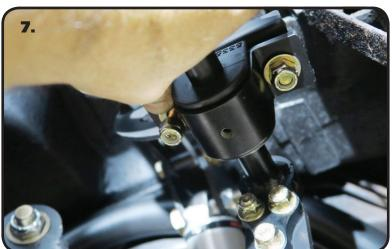
7. Insert the MuscleBar up into the car with the Arms pointing forward. Line up the holes in the Bushing Straps with the Bolts sticking down out of the mounts on the crossmember. While holding the bar in place, install a 3/8" Flat Washer and 3/8"-16 Nylok Nut on each of the (4) bolts sticking through the bushing straps. Torque the hardware to 45 ftlbs.
