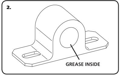
**2.** Apply Lithium grease to the inside of the sway bar bushings using the tube of grease supplied in the kit.
