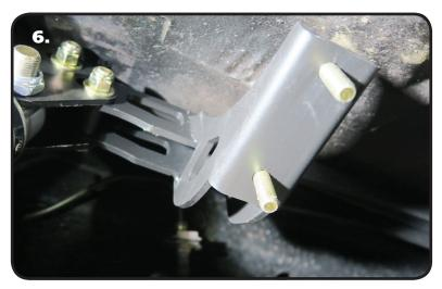
**6.** Install a 3/8" Flat Washer on each of (4) 3/8"-16 x 1 1/4" Bolts. Install (2) in each MuscleBar mount that is built into the rear shock crossmember. They will be installed with the threads pointing down to help simplify the MuscleBar installation.
