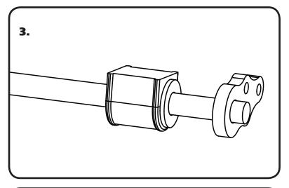
**3.** Install the Bushings by opening them up at the split and sliding them over the bar. They are positioned on the inside of the stop ring.
