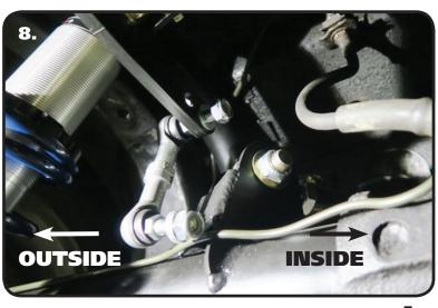
**8.** Install a 3/8" Flat Washer on the threads of one end of the PosiLinks. Insert the PosiLink into the OUTER hole of the musclebar arm with the threads pointing to the inside of the car. Refer to **Image 8**. Install a 2nd 3/8" Flat Washer on the inside of the arm followed by a M10-1.5 Nylok Nut. Repeat on the other arm with the threads pointing to the inside of the car. Torque the Nuts to 37 ftlbs.
