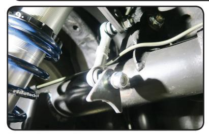
**9.** Attach an Axle Tab to the other end of the PosiLink. Use a 3/8" Flat Washer on each side of the tab. Install a M10-1.5 Nylok Nut and tighten enough to hold it in place. You will want to detach the PosiLink from the Tab for final welding.
