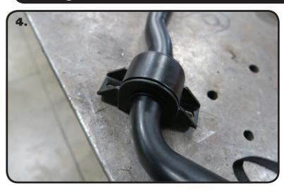
**4.** Install Bushing Straps Over the Poly SwayBar Bushings.
