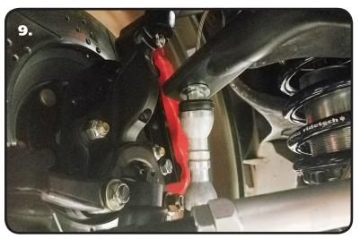
**7.** Insert one end of the PosiLink assembly into the hole in the T-bushing. Install a second T-Bushing up from the bottom of the control arm, sandwiching the control arm with the T-bushings. Install a M10-1.5 Nylok Nut on the threads of the PosiLink that is sticking through the t-bushings. Repeat steps 6 & 7 on the other side and tighten then nuts.
