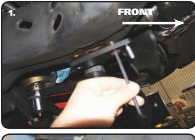
**1.** Attach the Adapter Plate to Frame positioned with the 3/8"-16 Stud to the Front of the Car and the Rear Hole aligned with the Rear OEM Hole. The Adapter Plate is attached to the Frame using a Flat Head Bolt and Red Loctite. The OEM Threaded holes can be either, 5/16"-18 or 3/8" -16, hardware is supplied for each. Apply Red Loctite to the proper Bolt and insert it through the Adapter. Thread the Bolt into the Front OEM Hole and tighten.
