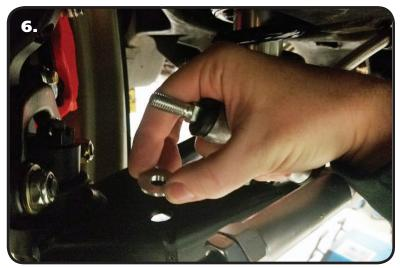
**6.** Insert a T-Bushing into the sway bar hole in the control arm. The SMALL diameter goes into the hole on the control arm.
