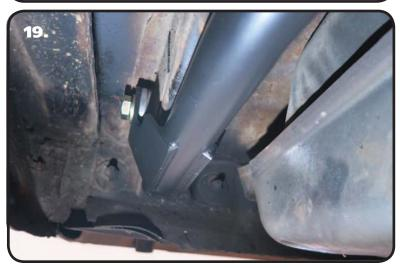
19. Attached the rear of the subframes to the newly installed Rear Frame Bushings. The kit includes a Driver and Passenger Subframe. Each one will be installed with the tabs to the inside of the car. Install a 5/8" Flat Washer on a 5/8"-11 x 4 1/2" bolt and insert it through the tabs and bushings with the threads to the inside of the car. With the bolt/washer installed, install a 5/8" Flat Washer and 5/8-11 Thin Nylok Nut on the threads sticking through. DO NOT TIGHTEN.
