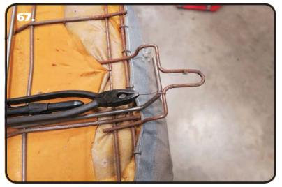
**67.** We used Safety Wire Pliers to twist the wires, but you can use regular Pliers or Vise-Grips to twist it. Grab the wire approximately 1" from the frame wire and twist it until it is tight. If you twist it too much, it will break. After twisting the safety wire, trim off some of the twisted part leaving approximately 1/2". Safety Wire the Frame Wire to the seat frame at every location circled in **Image 64**.
