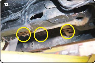
**12.** The front OEM leaf spring mount is attached to the body using u-nuts. New 3/18"-16 U-Nuts are supplied in the kit. Install the U-Nuts in place of the OEM u-nuts.
