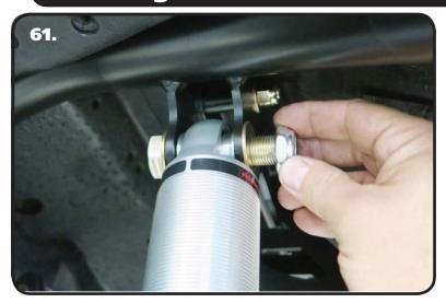
**61.** Insert the Shock with the 5/8" ID Spacers into the Shock Crossmember. Line up the holes in the crossmember with the spacers and shock bearing. Install a 5/8" Flat Washer on to a 5/8"-18 x 2 1/2" Hex Bolt, insert into the lined up holes. Install a 5/8" Flat Washer followed by a 5/8"-18 Thin Jam Nylok Nut. Torque to 75 ftlbs.
