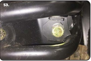
**53.** Use **Illustration 50** on Page 23 as a reference for installing the Indexing Washers. Install the Washers with the upper bar in the MIDDLE POSITION. The Outer Washer is installed with the hole forward. The Inner Washer is installed with the hole to the rear. The R-Joint is attached to the Bulkhead using a 5/8"-18 x 3 1/2" Hex Bolt & 5/8"-18 Thin Nylok Nut with a 5/8" Flat Washer on each side. Repeat on the other Bar. Torque the hardware to 75 ftlbs.
