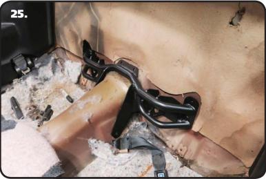
**25.** Set the Upper Bar Bulkhead in place over the driveshaft tunnel lining up the 2 lower holes with the 2 slots you just created.
