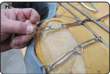
**71.** The Kit includes 2" Extension Rings to help with the longer span. It is necessary to Hog Ring 2 of the together to reach the wire with the seat cover. The idea is to keep the seat cover from coming loose.
