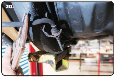
**20.** The front of the Subframes will swing up and engage onto the Bung on the Front Lower Mount as seen in **Image 21**. Later cars have the brake line mounted on the drivers rear frame rail, this will need to be clearanced to allow the Subframe to swing up in place. **Image 20** shows this mount.
