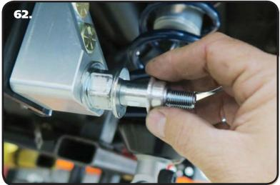
**62.** The Shock Stud requires spacers that are .400" long (90002067). Install a 5/8" ID 90002067 spacer **(Small side towards shock body)** onto the lower Shock Stud. Slide the bottom of the Shock onto the Stud. Install a second 5/8" ID 90002067 Spacer onto the Stud **(small side towards shock)**. You may need to jack the rearend up to Slide the Shock onto the Stud.
