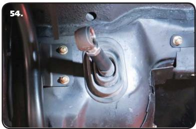
**54.** Slip the Rubber Boots over the Upper 4 Link Bars. Insert them into the cut holes. They install like a rubber grommet, they have a groove around the outside edge to nest the sheet metal into.
