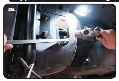
**39.** Depending on the year of your car, you may need to smooth out the outer edge of the upper 4 link bar hole to make the surface even. You can do this by inserting a solid object on the inside and hammering it smooth.
