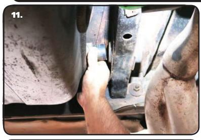
**11.** Remove the rear shackle bushings from the frame on both sides of the car. Clean the hole to remove any debris that may be in the hole.
