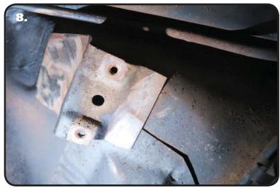
**8.** If your car has this style of exhaust bracket behind the axle, they will need to be cut off. Again, this can be done by drilling the rivets or cutting off flush with the tabs. The early cars have a different style of mount that doesn't need to be cut off.
