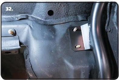
**32.** Removed the lower nut and washers from the Forward Subframe Tabs.
