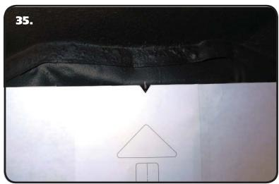
**35.** Use the Notch in the top of the Template to center it. Measure out from the frame rail on each side to find center. We found it easier to put a mark on the car, then align the template notch with the mark.
