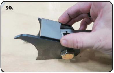
**50.** Set the Backer on the Tabs with the curved side toward the bolt. The flat side of the Backer needs to be positioned 1/4"-3/8 up from the bottom on the short side of the tabs. Center the Backer side to side and tack weld it in place. **Repeat this on the other set of tabs making a mirror image of the first**. Get both sets tacked together.
