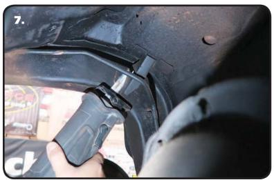
7. Cut the corner braces off that are located above the axle where the frame rail drops down. Depending on the year of your car, it may not be equipped with these braces. These can be removed by drilling the spot welds or cutting them of flush with the tabs.
