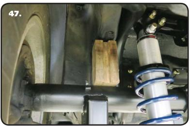
**47.** One helpful trick to help maintain ride height and pinion angle while positioning the differential is to put a spacer between the axle and the outside of the frame as shown in **Image 47**. This spacer should be 5 1/4" tall giving the Shockwave an eye-to-eye measurement of approximately 14 1/2". When measuring the axle center you can measure off of the frame rails. We also use a plum bob off the quarter panels to double check the axle center. Refer to Page 20 on Setting the Pinion Angle.
