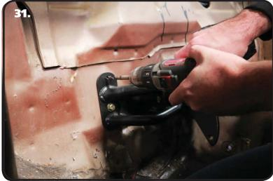
**31.** Drill the top 2 outer holes in the Bulkhead with a 3/8" Drill Bit. Install a 3/8" Flat washer on each of (2) 3/8"-16 x 1 1/4" Hex Bolts and insert them into the drilled holes.
