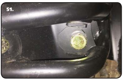
**51.** Use **Illustration 48** on Page 21 as a reference for installing the Indexing Washers. Install the Washers with the Setting Jig in the MIDDLE POSITION. The Outer Washer is installed with the hole forward. The Inner Washer is installed with the hole to the rear. The Setting Jig is attached to the Bulkhead using a 5/8"-18 x 3 1/2" Hex Bolt & 5/8"-18 Thin Nylok Nut with a 5/8" Flat Washer on each side.
