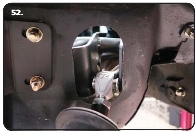
**52.** Verify the Spacers are installed in the R-Joints of the Upper Bars. Insert the Upper Bar through the hole cut previously. The R-Joint will insert into the Bulkhead aligning the though hole with the slots in the Bulkhead.
