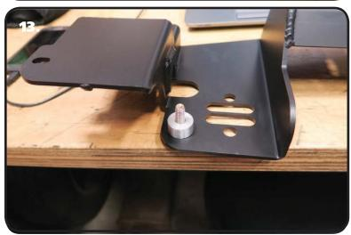
**13.** Insert a 3/8"-16 x 1 1/2" Hex Bolt in the rear hole of the Lower Bar/Subframe Mount. This needs to be inserted from the bottom with the threads sticking up. Install the Aluminum Spacer on the bolt.
