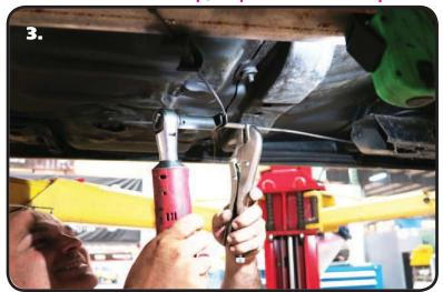
**3.** Disconnect the emergency brake cables from the main cable at the adjuster. It is located under the driver side rear foot well. After it is removed, disconnect the cables from the connector that joins the rear cables together. Set the hardware and connector aside, you will need them for reassembly.
