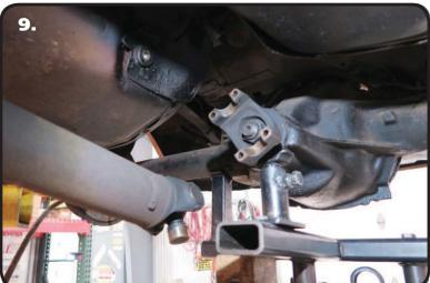
**9.** Remove the U-joint straps from the yoke. Disconnect the driveshaft from the rear differential. It is a good idea to wrap masking tape around the end of the driveshaft to help keep the u-joint caps in place.
