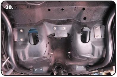
**38.** Use a straight edge to draw a reference line from circle to circle. You will be cutting out the rest to make an obround. **Image 38** shows both sides cut out. After connecting the holes, remove any burrs from the edge of the holes. Install a 3/8" Flat Washer & 3/8"-16 Nylok Nut on each of the 4 bolts sticking through the Forward Tabs that were installed previously. **DO NOT TIGHTEN THESE 4 BOLTS AT THIS TIME, THEY WILL GET TIGHTENED AFTER THE SHOCK CROSSMEMBER IS INSTALLED.**
