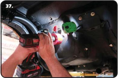
**37.** Drill the center punched spots with a 3" hole saw.
