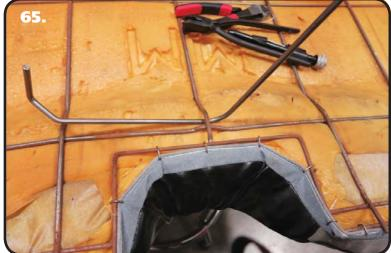
**65.** The Frame Wire needs to be inserted under the middle wire, right about the first LONG horizontal frame wire. It will lay on top or beside of other frame wires.
