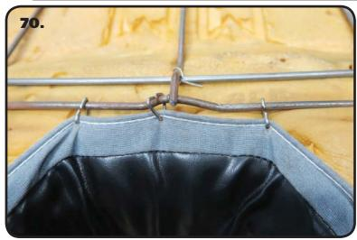
**70.** The kit includes Hog Rings and Extensions to attach the seat cover to the frame. The center can be pulled up to the wire above it and attached with Hog Rings.
