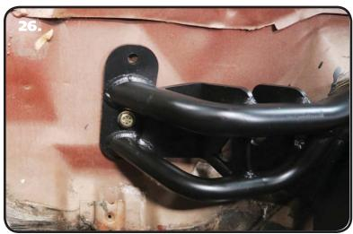
**26.** Install a 3/8" Flat Washer on each of (2) 3/8"-16 x 1 1/4" Hex Bolts. Insert a bolt/ washer into the lined up lower holes. Install a 3/8" Flat Washer & 3/8"-16 Nylok Nut on bolts where they come through the forward tab of the subframe. Lightly tighten the bolts.
