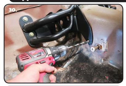
**30.** The Bulkhead has a tab the goes forward on each side of the driveshaft tunnel, in the end of each tab is a 1/2" hole. Using the Bulkhead holes as a template, drill the driveshaft tunnel with a 1/2" drill bit. Do this for the forward hole in each tab. Insert the supplied 1/2"-13 x 1 1/4" bolt in each drilled hole with a 1/2" washer on the top side and bottom side, follow the bottom washer with a 1/2"-13 Nylok Nut. Torque the 2 bolts/nuts to 110 ftlbs.
