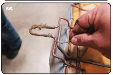
**66.** The kit includes (6) long pieces of Safety Wire. Cut the long pieces in about 3" pieces. We will start in the location close to the attaching loop. Start by wrapping a 3" piece of Safety Wire around the Frame Wire and seat frame close to the 1st bend of the frame wire. Twist it a little to hold it in place.
