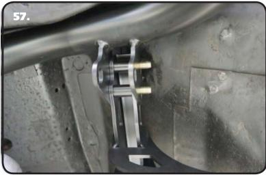
**57.** Install a 3/8" Flat Washer on each of (4) 3/8"-16 x 2 1/4" Hex Bolts. Install a Bolt/Washer in each of the (4) mounting holes. With the Bolts installed, install a 3/8" Flat Washer and 3/8"-16 Nylok Nut on each of them. Torque to 45 ftlbs. **ALSO TORQUE THE 4 BOLTS TO 45 FTLBS THAT WERE LEFT LOSE IN STEP 38.**
