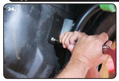
**24.** Use a die grinder, or similar tool, to slot the lower hole of the forward tabs. Use the Tab as a template for slotting the hole.
