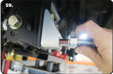
**59.** Installing the Shock Stud into the Lower Mount. Install a 5/8" Flat Washer onto the 5/8"-18 threads of the shock stud. Apply Red Loctite to the 5/8" threads of the stud. Thread the Shock Stud into the threaded hole of the Lower Mount. Repeat on both sides and torque the Shock Stud to 65-75 ftlbs.
