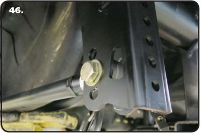
**46.** Insert the Lower Bar R-Joint into the Lower Axle Bracket. Line the through hole of the R-Joint with the MIDDLE set of holes of the Axle Bracket. Install a 5/8" Flat Washer on to a 5/8"-18 x 3" Hex Bolt, insert into the lined up holes. Install a 5/8" Flat Washer followed by a 5/8"-18 Thin Jam Nylok Nut. Repeat on both sides and tighten the Bolts/Nuts enough to eliminate any gaps..
