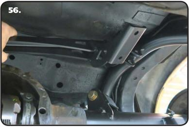
**56.** Insert the Shock Crossmember into the tabs on the Subframe. It is installed with the Swaybar Mounts to the REAR of the car. There are (2) mounting holes on each side that line up with the slots in the Subframe Mounts.
