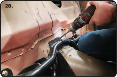
**28.** Drill the top 2 holes in the Bulkhead with a 3/8" Drill Bit. Install a 3/8" Flat washer on each of (2) 3/8"-16 x 1 1/4" Hex Bolts and insert them into the drilled holes.
