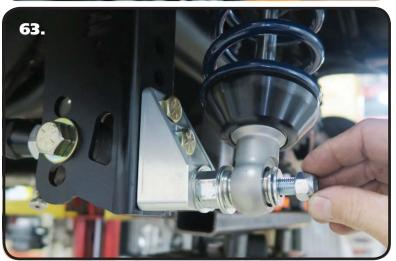
**63.** Install the 7/16" Flat washer and 7/16" Nylok nut. Tighten the upper and lower shock bolts. Torque the Upper Bolt to 75 ftlbs and the Lower Nut to 40 ftlbs. The designed ride height of the CoilOver/Shockwave is 14 1/2" center to center.
