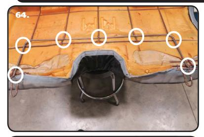
**64.** The rear seat frame will need to be modified to clear the bulkhead. A new Frame Wire is included to help stiffen the seat. Safety Wire is included to wire the Frame Wire to the existing seat frame. **Image 64** has circles around the area that will need to be safety wired. You will also notice that part of the OEM seat frame has been cut out, we will show you where to cut it.
