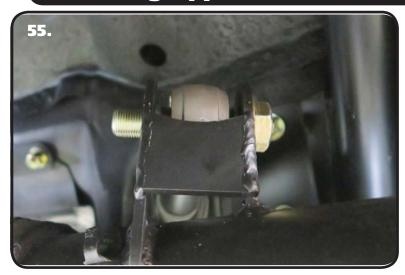
**55.** Verify the Spacers are installed in the R-Joints of the Upper Bars. Insert the R-Joint into the upper bar mount of the rear differential. Install a 5/8" Flat Washer on to a 5/8"-16 x 3" Hex Bolt. Line up the holes in the axle tabs with the through hole of the R-Joint, insert the bolt/washer from the OUTSIDE with the threads pointing inward. Install a 5/8" Flat Washer followed by a 5/8"-18 Thin Jam Nylok Nut. Repeat on both sides and tighten the Bolts/Nuts enough to eliminate any gaps.
