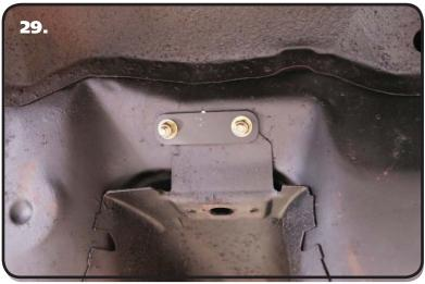
**29.** Install the supplied Backer Plate on the bolts sticking through the floor pan. Install a 3/8" Flat Washer & 3/8"-16 Nylok Nut on each bolt. Torque to 45 ftlbs.
