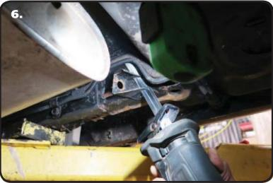
**6.** Remove the emergency brake cable bracket from the frame. You can do this by drilling out the spot welds or cutting it flush with the frame rails. We used a sawzall to remove them.
