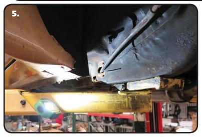
**5.** Remove the bracket on the outside of the frame that holds the emergency cable in place. This will allow the cable to be pulled out of the car. You do NOT need to remove the cables from the differential.
