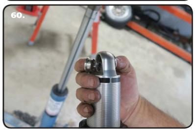
**60.** Ridetech CoilOvers or ShockWaves require a spacer on each side of the bearing. The Upper Crossmember uses a 5/8" ID spacer that is 3/8" long (90002042). The overall width with a spacer on each side will be 1 1/4". **The small side of the spacer goes towards shock bearing.**
