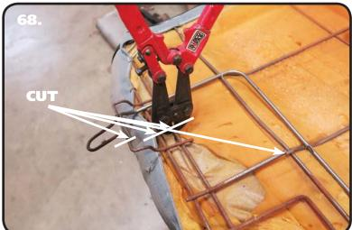
**68. Images 68 & 69** illustrate where to cut the OEM seat frame. The BOTTOM 3 horizontal wires get cut in-line with the end of the Frame Wire. The 3 CENTER vertical wires get cut below the 1st horizontal wire that runs the width of the seat. We used a bolt cutter to cut them, but the can be cut with a saw. You will need to disconnect any hog rings that attach the seat cover to the area being removed.
