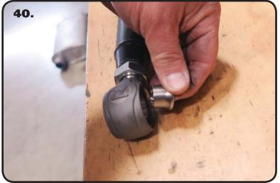
**40.** The 4 Link Bars in this kit are equipped with R-Joints. The R-Joints require spacers to be installed in them. Insert a Spacer into each side of the R-Joints. The Spacers are installed into the R-Joint with the small diameter going into the center pivot ball. Push them in until they stop.
