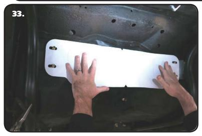
**33.** Cut the 4 Outer Slots out of the template. Slide it over the 4 bolts sticking through the Forward tabs. Make sure the ARROW POINTS UP!
