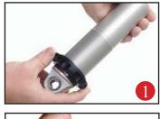
First using the supplied lower adjuster nut(90002222) thread the nut onto the shock from the bottom side as seen in figure 1
