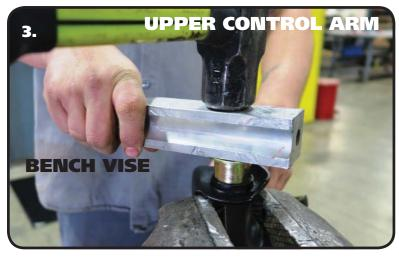
**3.** Use another Piece of Metal or Strong Wood to Drive the Outer Shell into the Control Arm until the Shell stops against the Control Arm.
