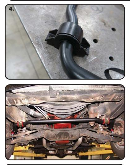
6. SWAYBAR CONTROL ARM **4.** Install Bushing Straps Over the Poly SwayBar Bushings.
