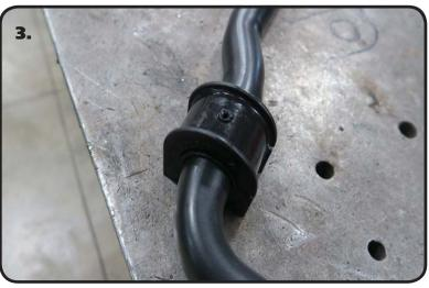
**2.** The Delrin Liner is split on one side to ease installation. We found it easier to install by opening up the Liner enough to slide it onto the end of the SwayBar, then sliding it into position. It will open up and slide over the curves in the Bar. Install a Liner on each side of the SwayBar in the approximate location they will need to be when installing the SwayBar on the Car.
