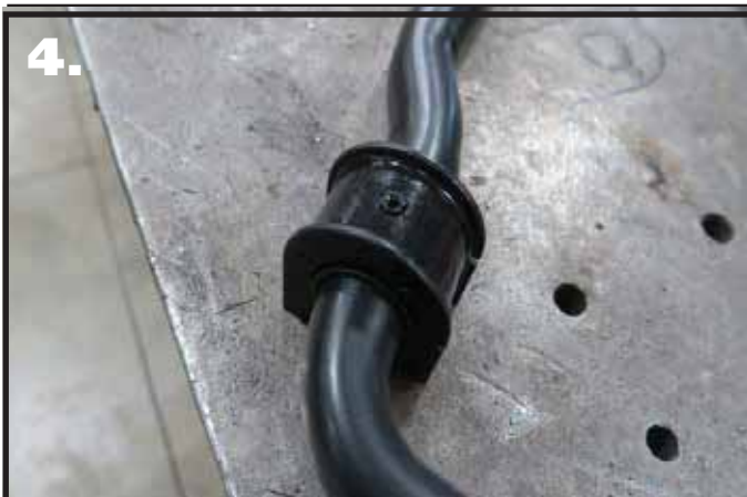
4. Open the sway bar bushing at the split and slip it OVER the sway bar. Do this for both bushings.
