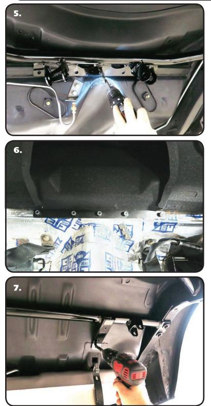
**5.** Image 5 shows how the Front Tab overlaps the body seam. Multiple pieces of the car body overlap at this joint making it a strong area to attach to. Drill these 5 holes with a 3/8" drill bit using the cradle as a template.
