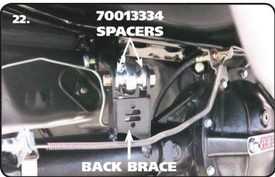
**20.** One helpful trick to help maintain ride height and pinion angle while adjusting is to tack weld a spacer between the axle and the outside of the frame as shown in the picture. This spacer should be 8 1/2" tall giving the Shockwave an eye-to-eye measurement of approximately 14 1/2". When measuring the axle center you can measure off of the frame rails. We also use a plum bob off the quarter panels to double check the axle center. Refer to Page 11 on Setting the Pinion Angle.
