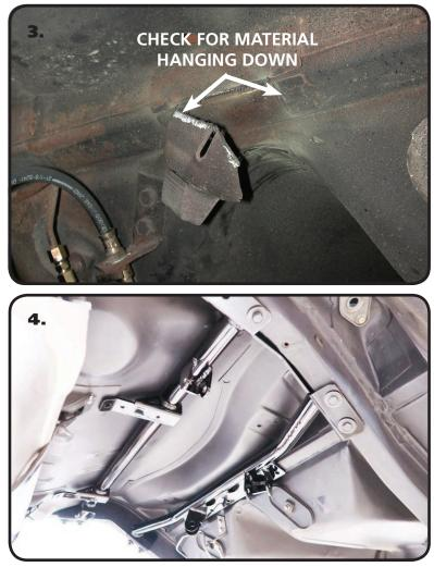
**3.** Remove the Factory Pinion Snubber and Mount from the car, this is necessary for clearance of the Upper Cradle. We use a cut off wheel to remove the mount. Make sure the area where the ARROW is pointing has no material sticking down. The tabs that are against the body can remain. Check both sides where the snubber mount attached to the body.
