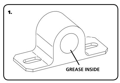
**1.** Apply Lithium grease to the inside of the sway bar bushings using the tube of grease supplied in the kit.
