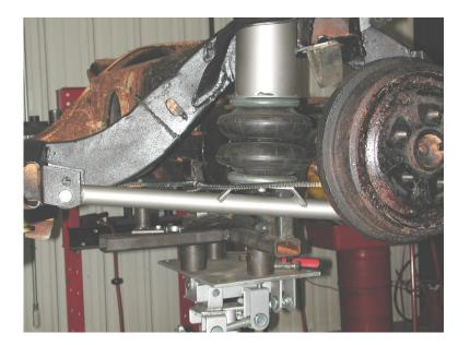
10. Fasten the air spring to the lower StrongArm using a 3/8" x 3/4" bolt, lock washer and flat washer.
