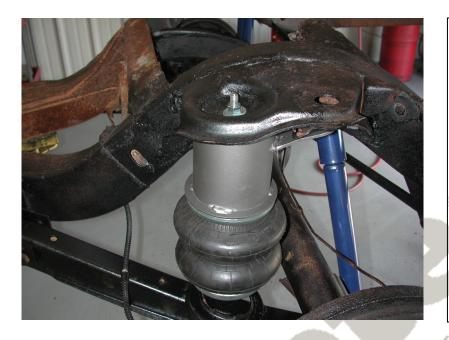
3. Apply thread sealant to the air fitting and screw it into the top of the air spring.
